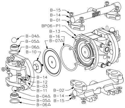
Torque Requirements: B-10: 7.0-8.0 Nm
